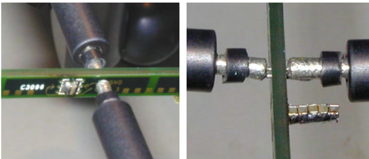
Figure 45. Small fixture with one and five stacked capacitors on the pads.
