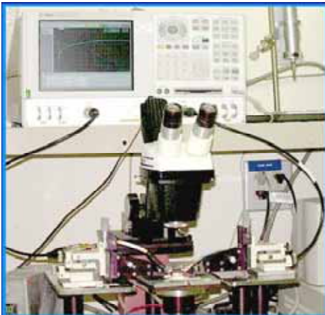
Figure 1. Data acquisition equipment includes a network analyzer, pico-probes and a high frequency test substrate.
