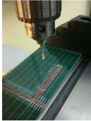
Figure 20 Photograph of the milling machine and secured board. Careful adjustments and measures were taken which allowed the board to be milled in approximately one-mil increments.
