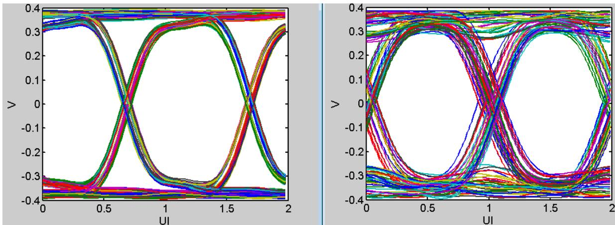
Figure 12 Simulated eye (left) vs measured eye (right) at FDR
