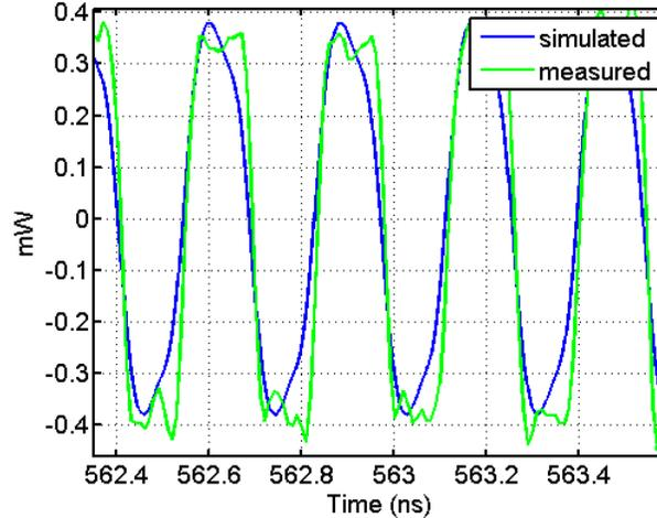
Figure 17 EDR MBOM optical output measurement vs simulation
