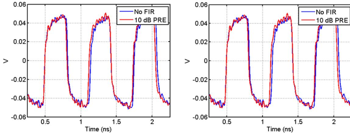
Figure 15 Varying pattern generator FIR settings and observing effect on MBOM electrical output
