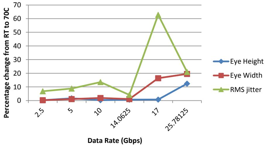
Figure 19 Measurement of MBOM electrical output parameters at room temperature (RT, 25°C) and high temperature (70°C)
