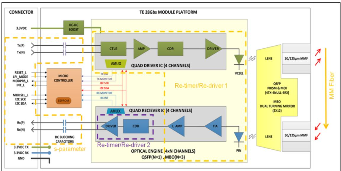
Figure 1 Block diagram of MBOM in optical loopback
