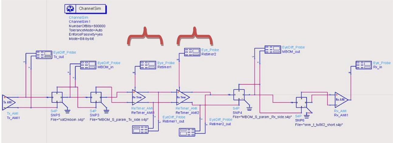
Figure 8 Block diagram showing simulation setup. First and second MBOM stages highlighted with brackets
