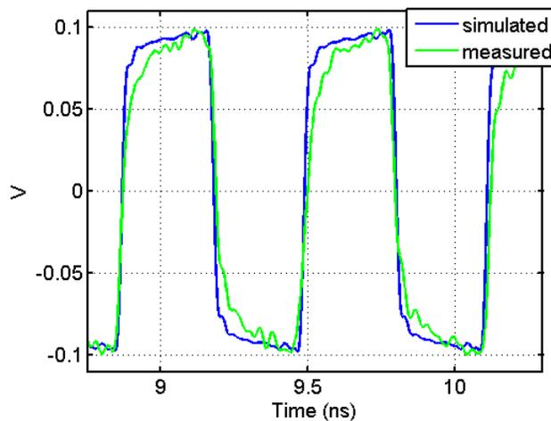
Figure 14 Measurement vs simulation of MBOM electrical output to a clock pattern slowed by a factor of 16. Minimum output amplitude, minimum pre-emphasis, and maximum CTLE settings
