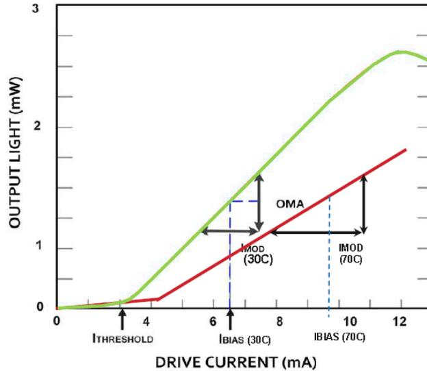
Figure 18 VCSEL input-output curve with varying temperature
