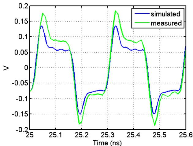
Figure 13 Measured vs simulated waveform of MBOM electrical output at FDR
