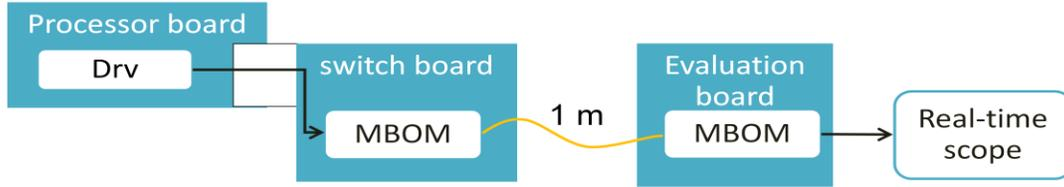
Figure 6 Measurement setup for FDR
