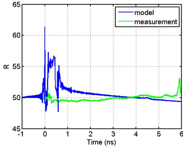
Figure 10 TDR of evaluation board traces and connectors from model and measurement
