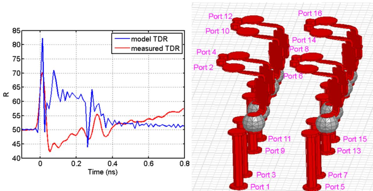
Figure 9 TDR of MBOM socket from measurement and model (left). Diagram showing MBOM socket 3D model (right)
