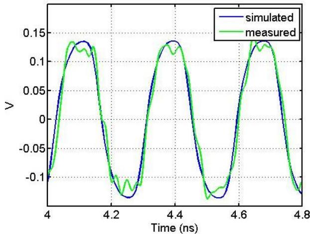
Figure 11 MBOM input electrical signal measurement to simulation correlation
