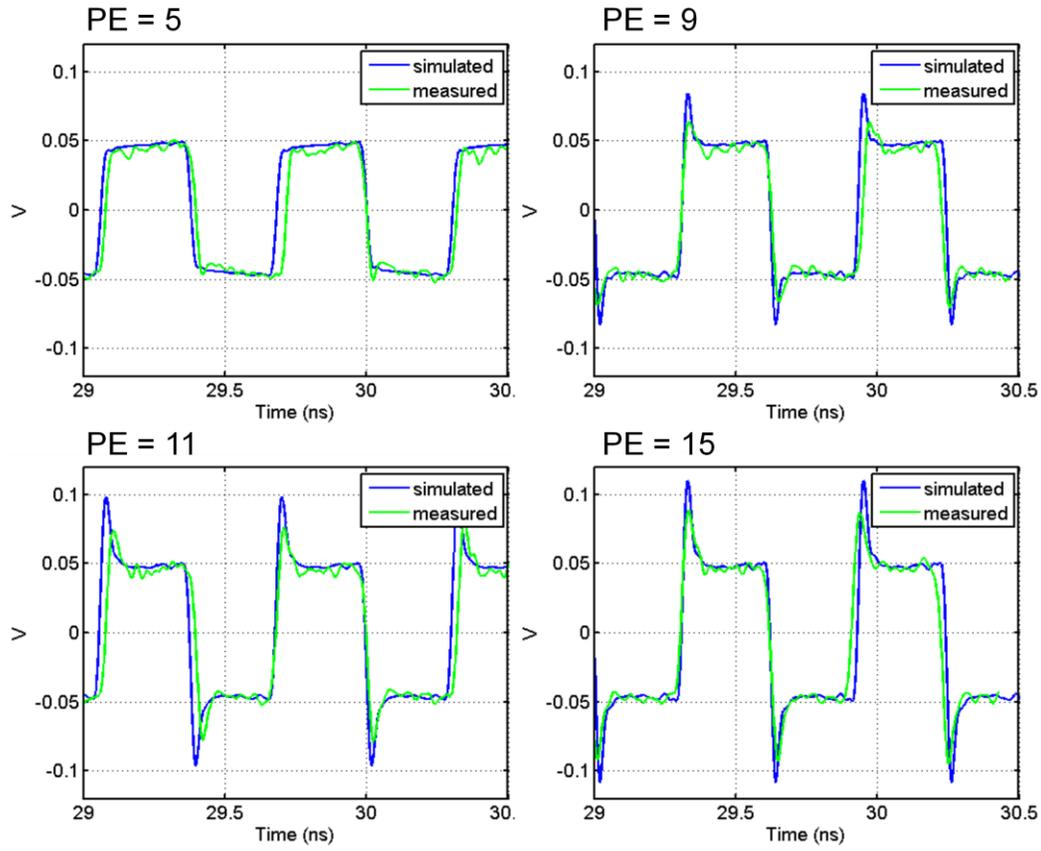
Figure 16 Measurement and simulation correlation for various MBOM pre-emphasis (PE) values
