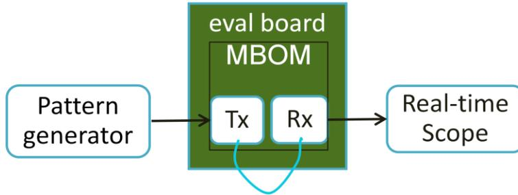
Figure 7 Measurement setup for EDR
