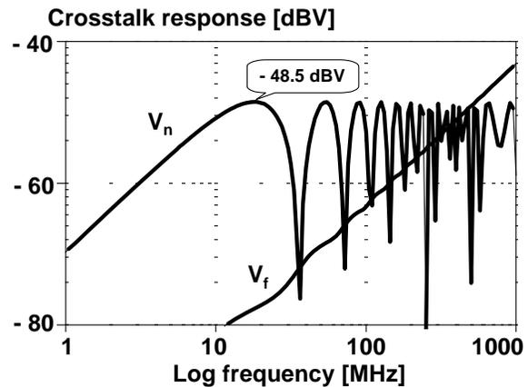
Figure 3.: Simulated crosstalk response of the reference structure with two outer traces and matched terminations. Source voltage for time-domain response: 0-to-2 V piece-wise linear ramp. Source voltage for frequency-domain response: 2 V<sub>rms</sub> sinewave.
