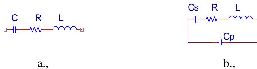
Figure 1: Lumped equivalent circuit of bypass capacitors with their parallel DC leakage resistance neglected. Figure 1(a) is valid for low and medium frequencies, (b) is good for higher frequencies. All parameters are treated as variables of frequency.
