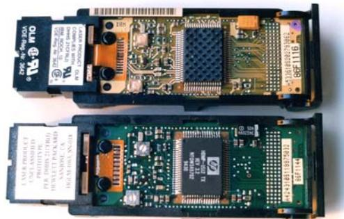
*Figure 2: An early prototype of the 1.0625 Gbps FibreChannel media-interface board.*
