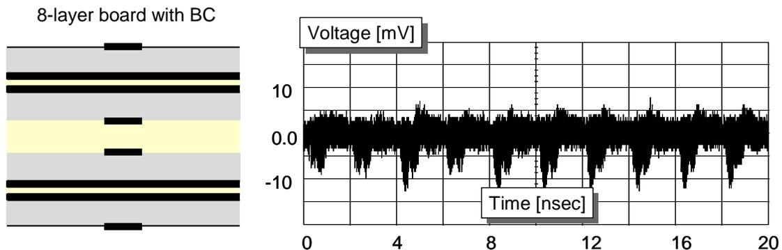
*Figure 3: Stack-up and measured noise on the supply rail.*
