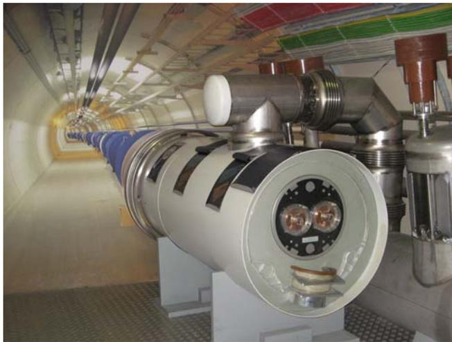
**Figure 1:** A cross section view of the LHC experiment, where two particle beams are kept on counter-rotating paths by a network of superconducting magnets.
