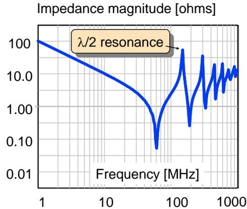
**Figure 2:** Measured impedance magnitude of a 480 x 110 mm rectangular parallel plate pair with 1.5mm FR4 dielectric separation.
