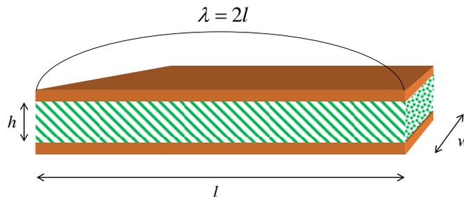
**Figure 1:** A pair of metal layers forms not only a parallel-plate capacitor, but also a two-dimensional resonator.
