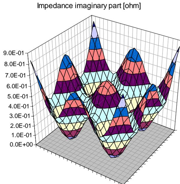
**Figure 3:** Simulated imaginary part of impedance of a 25x25cm plane pair with open boundaries, separated by 50um of FR4 dielectric separation. Impedance surface is shown at 533 MHz.
