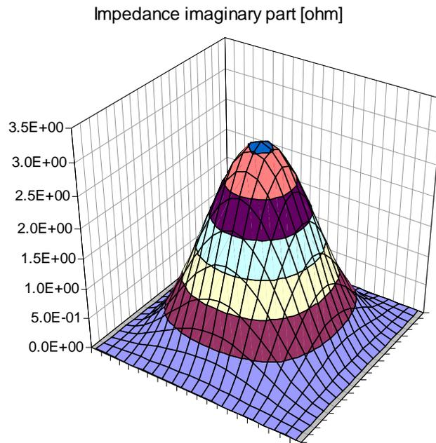
**Figure 4:** Simulated imaginary part of impedance of a 25x25cm plane pair with shorted boundaries, separated by 50um of FR4 dielectric separation. Impedance surface is shown at 383 MHz.
