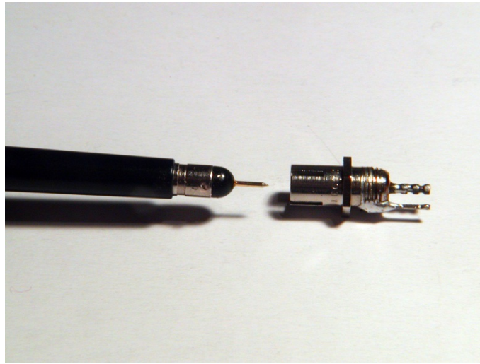
Figure 3: High-impedance passive probe with coaxial receptacle.
