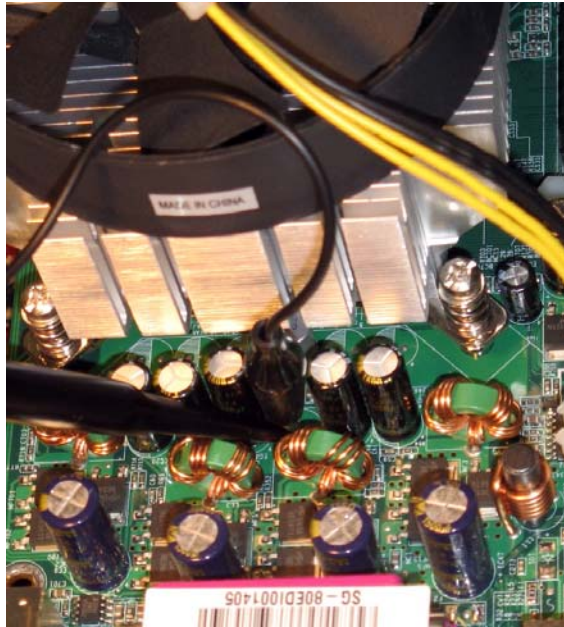
Figure 6: Connection of the high-impedance passive probe to the test site on the top side of the board.
