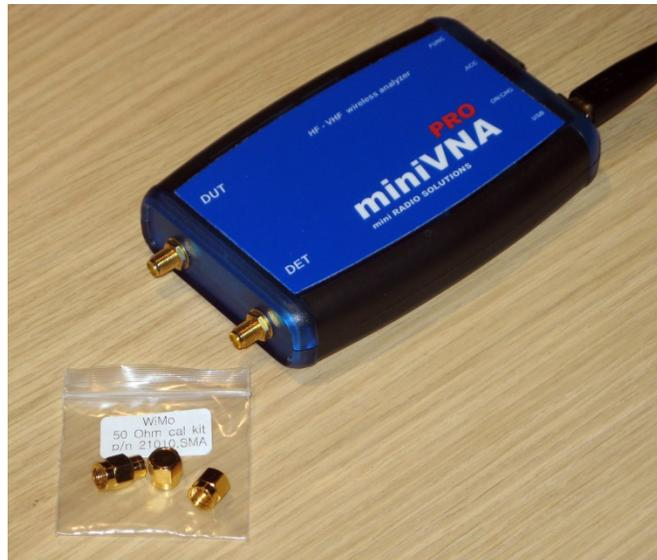
**Figure 1:** The USB-connected miniVNA Pro pocket-size VNA.
