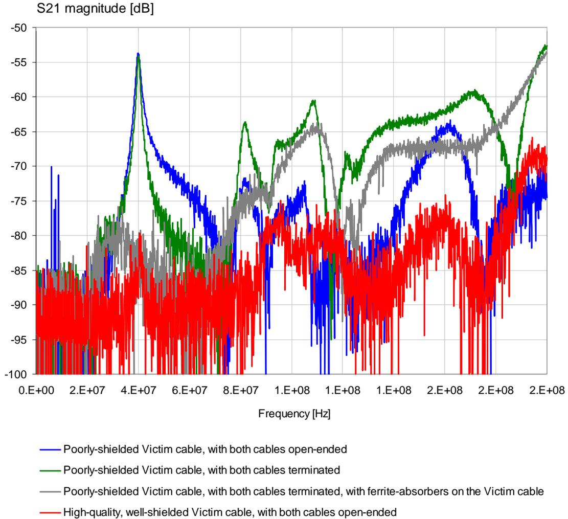
**Figure 4:** Crosstalk through the cable braid and air for four different cable combinations.
