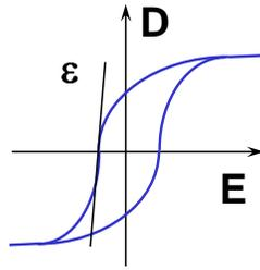
**Figure 2:** Relationship between the  $E$  and  $D$  fields in ferroelectric materials.
