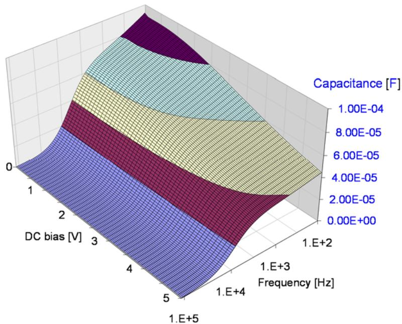
**Figure 3:** Capacitance as a function of frequency and DC bias. Measured on a 100 uF 4V Class 2 MLCC part.
