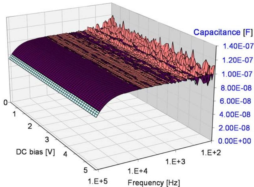
*Figure 4: Capacitance as a function of frequency and DC bias. Measured on a 0.1 uF Class 1 MLCC part.*
