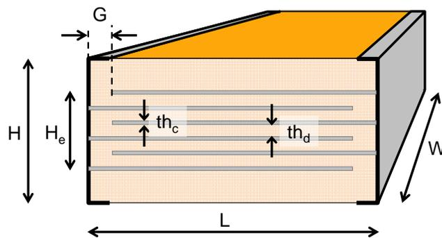
*Figure 1: Approximate internal geometry of MLCC.*
