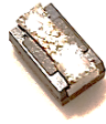
Figure 3.: Photo of a D-size Short reference piece. This is a D-size capacitor with a metal strip across its terminals.
