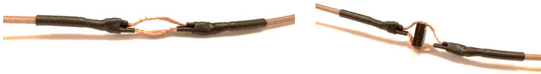
Figure 1.: Photo of solder-wick fixture (left) and a D-size capacitor in the fixture (right).
