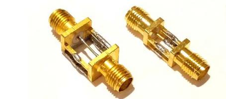
*Figure 2: Wide-base and narrow-base empty SMA fixtures.*
