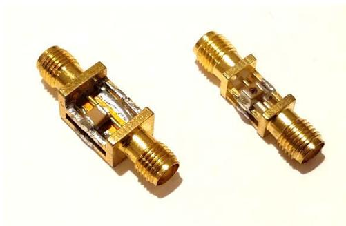
*Figure 3: Wide-base and narrow-base SMA fixtures with bypass capacitor.*
