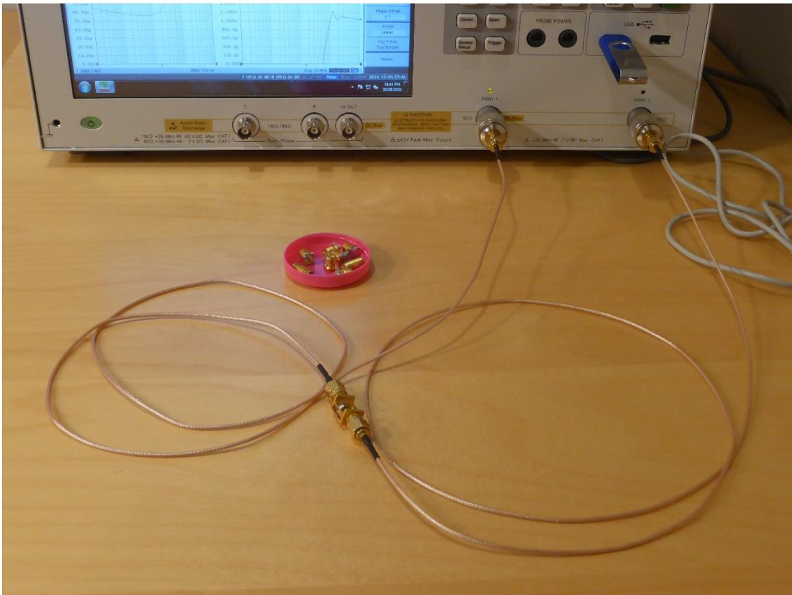
**Figure 4.:** Measurement setup with network analyzer and a back-to-back SMA fixture. E5061B loaner VNA is courtesy of Keysight.
