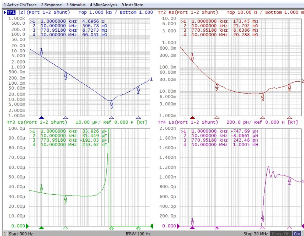
**Figure 5.:** Measurement data of a 47  $\mu\text{F}$  1210 size ceramic multi-layer capacitor taken in a setup similar to the one shown in Figure 4. E5061B loaner VNA is courtesy of Keysight.
