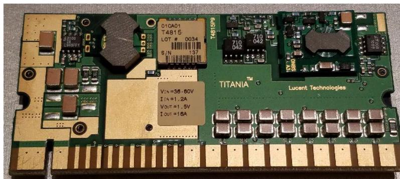
*Figure 5: A Lucent Technologies 16A DC-DC converter.*
