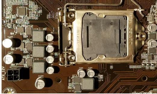
*Figure 2: Partial top view of a Gigabyte H110M-A motherboard.*
