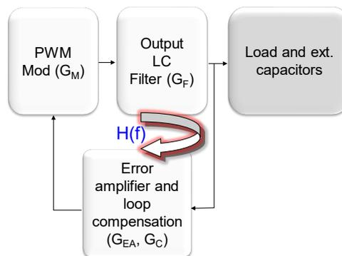
**Figure 4:** Block diagram of a switching voltage regulator.
