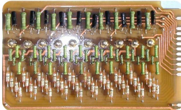
**Figure 1:** *A DTL (Diode-Transistor-Logic) from the early days of computers. You can notice that there is no power distribution component whatsoever on the board.*
