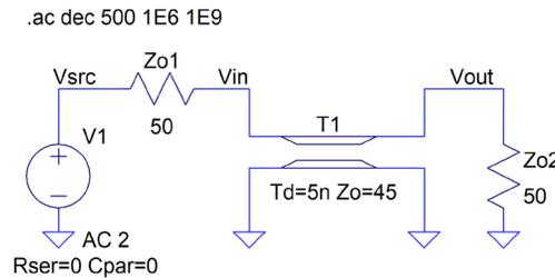
**Figure 2:** LTSPICE simulation circuit with impedance mismatch.
