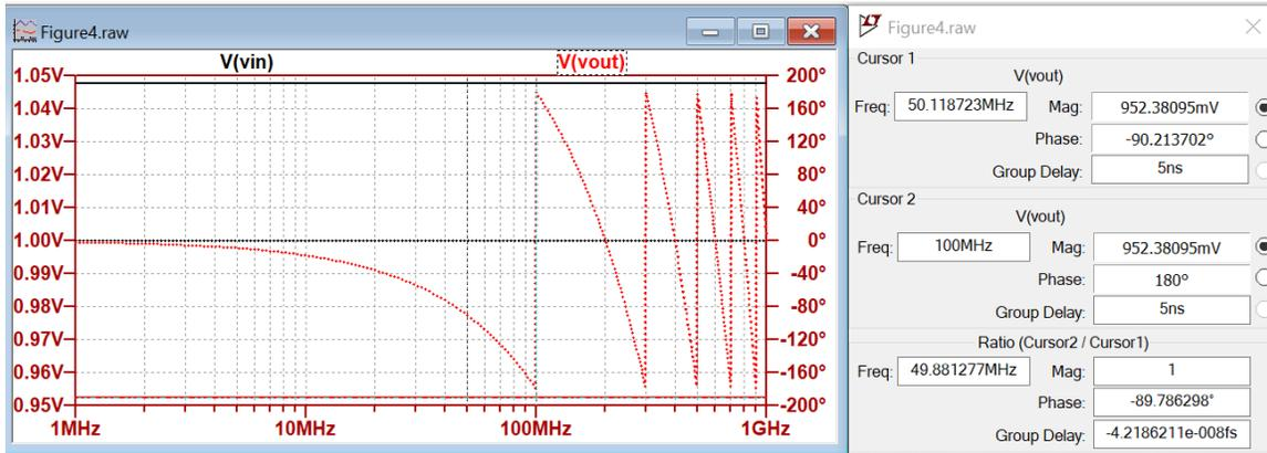
**Figure 5:** Frequency response of circuit in Figure 4. Voltage magnitudes are solid lines referencing the left vertical axis, phase is dotted line, referencing the right vertical axis.
