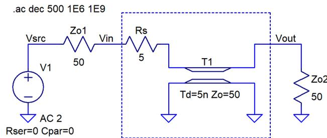
**Figure 4:** LTSPICE simulation circuit with series loss resistance represented by a 5-ohm series resistor.
