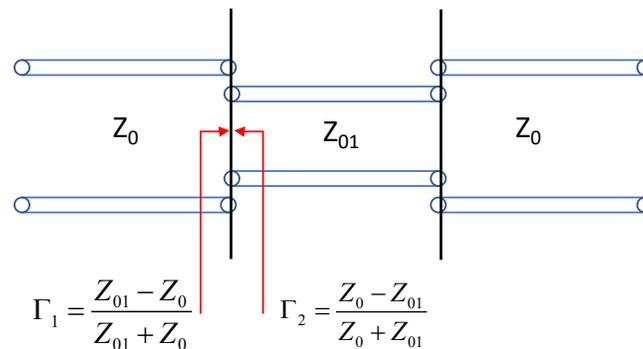
**Figure 1:** Definition of voltage reflection coefficient.
