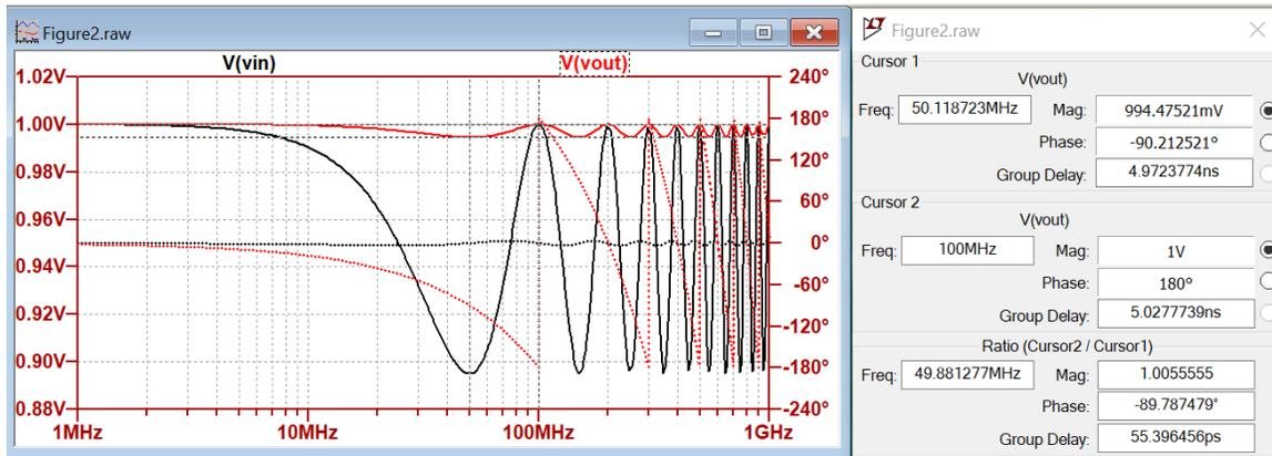
**Figure 3:** Frequency response of circuit in Figure 2. Voltage magnitudes are solid lines referencing the left vertical axis, phase is dotted line, referencing the right vertical axis.
