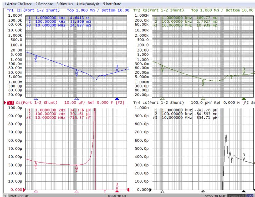
Figure 6.: Measurement data of the 47uF 1210 size ceramic multi-layer capacitor taken in the co-planar fixture.
