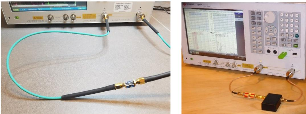
**Figure 4.:** Measurement setup with Keysight E5061B network analyzer. The common-mode toroid transformer on the right photo is encapsulated in a small black plastic box.
