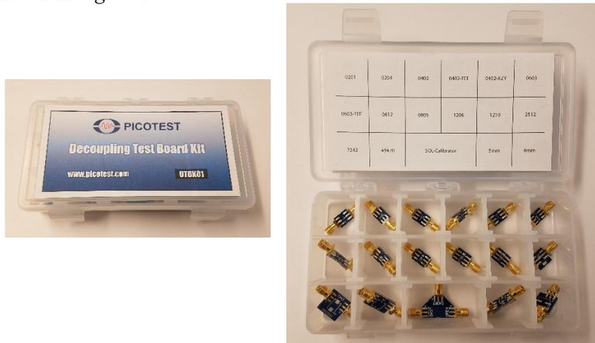
*Figure 1.: Picotest component characterization fixtures.*
