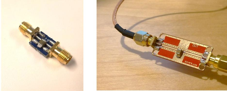
**Figure 5.:** 1210 size MLCC parts soldered on the PCB fixtures. 330uF 4V part on the left, 47uF 16V part on the right.
