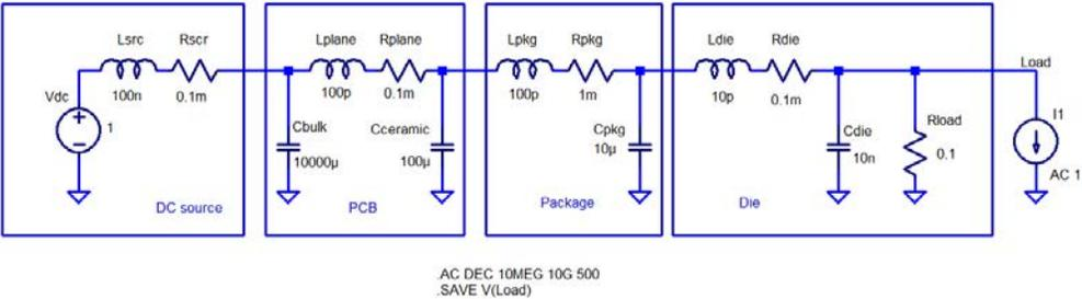
**Figure 1.:** LTSPICE schematics of a simple PDN.
