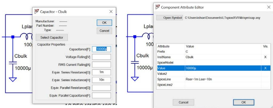
**Figure 4.:** Options to enter parasitic values for capacitors in LTSPICE.
