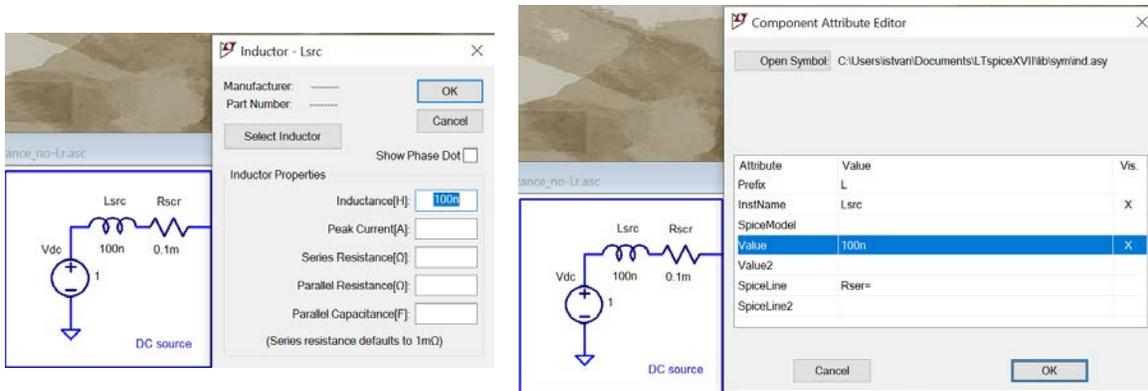
**Figure 7.:** Parasitic definitions of the Lsrc inductor.
