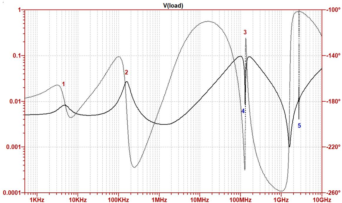
*Figure 2.: Impedance magnitude and phase of the simple PDN showed in Figure 1.*
