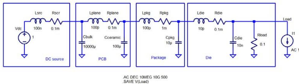
*Figure 1.: LTSPICE schematics of a simple PDN.*
