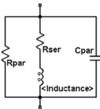
**Figure 6.:** Equivalent circuit of inductor parasitics and attribute list.
