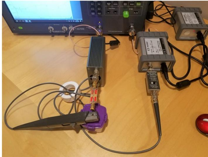
This image above shows a current measurement setup with a temporary loaner E5061B network analyzer (courtesy of Keysight) with a Tektronix P6021 clamp-on current probe. The test signal is boosted with a Juntek DPA-2698 dual DC-10MHz power amplifier (this is the rectangular box -with striped top- connected to Port1 of the VNA), while the output signal of the current clamp is boosted with a Picotest J2180A-20 low-noise preamplifier loaner (courtesy of Picotest).
