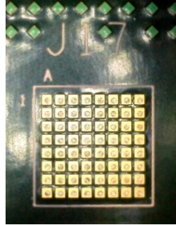
Figure 7: 8x8 via array on Section1 through Section5.
